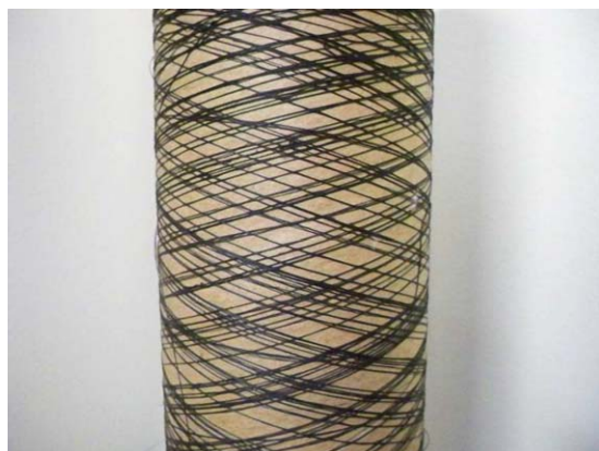
Figure 3. Bobbin of spun alginate doped with IONP. [Color figure can be viewed in the online issue, which is available at wileyonlinelibrary.com .]
